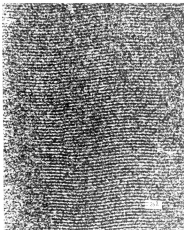
Figure 10. High-resolution electron micrograph showing final stages in development of undulating smectic planes in main-chain/side-group liquid crystal polymer.
