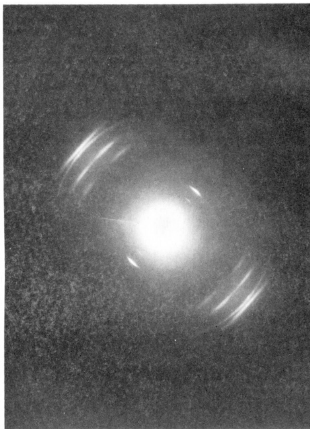
Figure 13. Diffraction pattern obtained from corresponding pure main-chain liquid crystal polymer.
