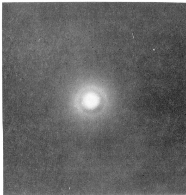
Figure 12. Diffraction pattern obtained from corresponding pure side-chain liquid crystal polymer.
