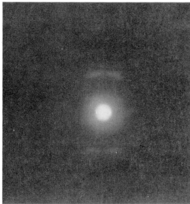
Figure 5. Electron diffraction pattern of main-chain/side-group liquid crystal polymer showing sharp small-angle reflections and oriented splitted wide-angle halo.
